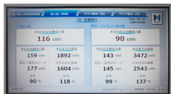
Energy management tool (Hulic Asakusabashi Building)
